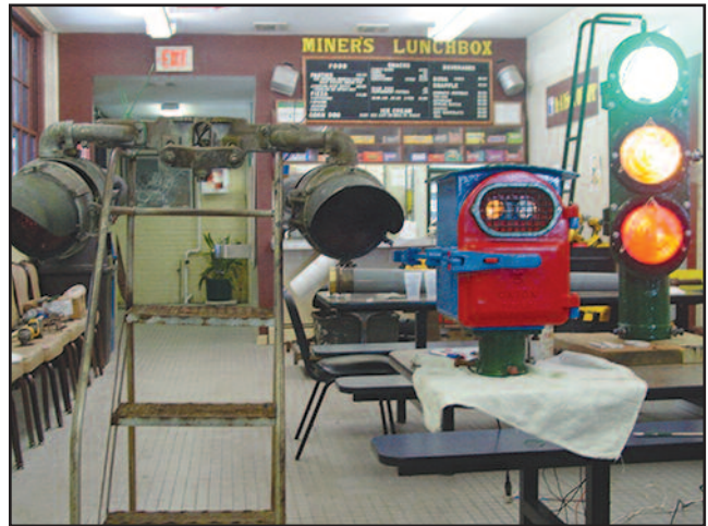
The Gift Shop is a comfortable area for working on our signals. Here you can see the completed block signal and illuminated signal box (right and center). The highway crossing flashing signal (left) is awaiting power-washing and paint stripping.
