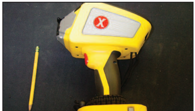
About the size and weight of a battery-powered drill, the XRF analyzer is truly portable and simple to use. Just aim and pull the trigger.
