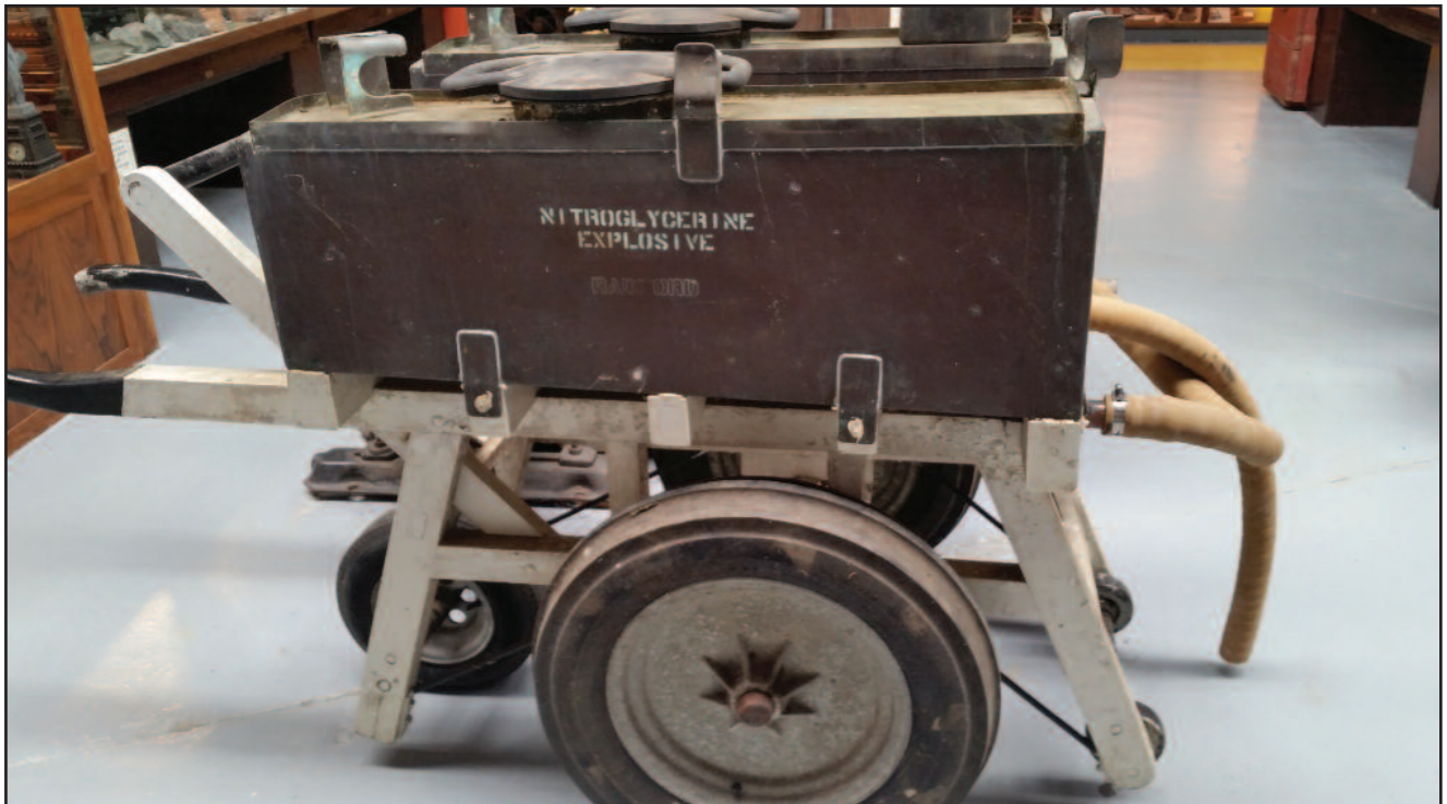
The "Nitro Buggy" was used to transport batches of nitroglycerin. Rather than risk a mishap in a pipeline that could destroy a large area of the complex (as the pipe would act as a fuse), isolated batches of nitroglycerine were transported on these special wooden carts. Note the large air-filled rubber tires to cushion the cargo.
